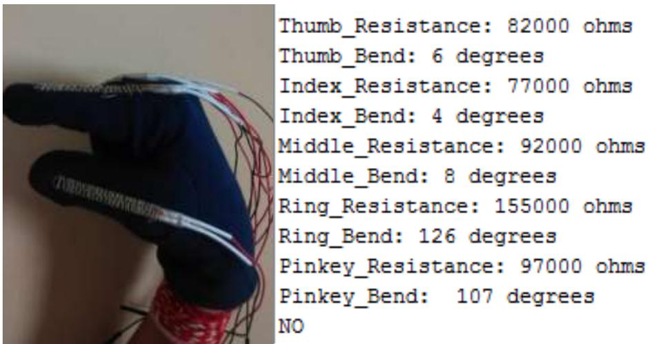
**Figure VI: Gesture and corresponding readings for message ‘NO’**
