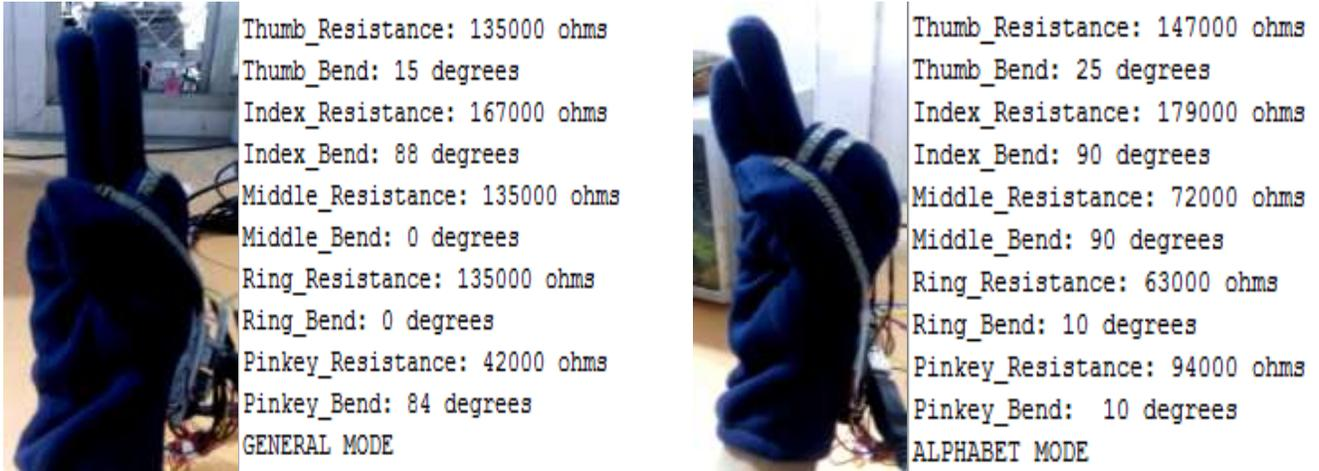
Figure IV: Gesture and corresponding readings for Mode Switching
