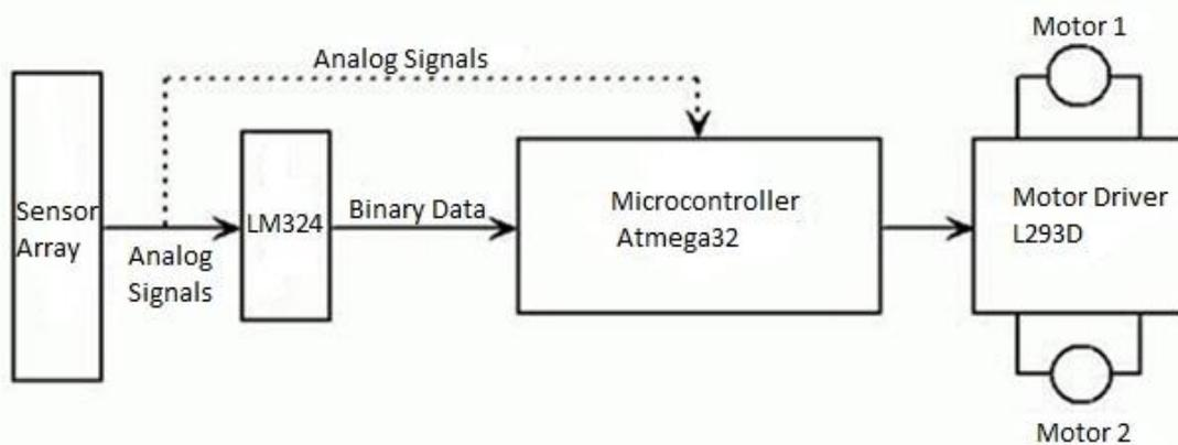
**Figure 1.** Block diagram of industrial fire fighting robot
