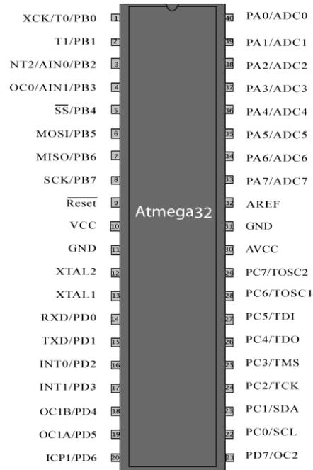
**Figure 3:** Pin diagram of Atmega 32
