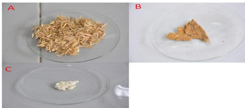
Figure-IV Optical photographs (A) RH (B) Alkali treated RH (C) Cellulose
