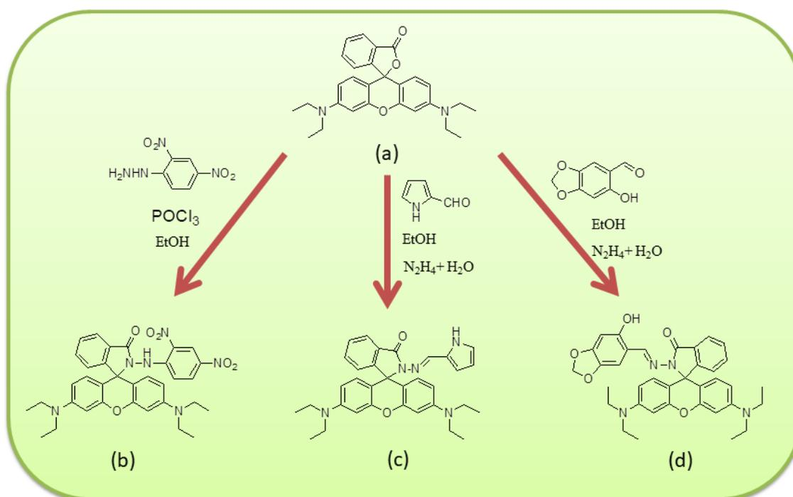
Figure-III Synthesis of chemosensors
