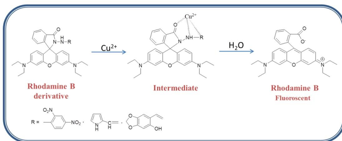
Figure-IV Binding mechanism of  $\text{Cu}^{2+}$  with different chemosensors
