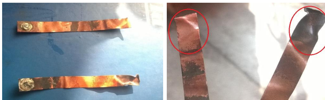
Figure – VII (a) Electrodes before electrolysis (b) Electrodes after electrolysis
