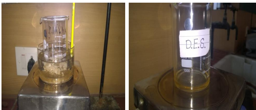
Figure - II (a) Apparatus set-up for synthesizing \text{ZnCl}_2 -Acetamide DES (b) Synthesized DES
