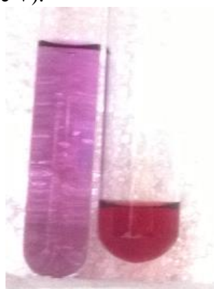
Figure - V: On the left , blue litmus solution. On the right , blue litmus solution turned red in presence of DES.
